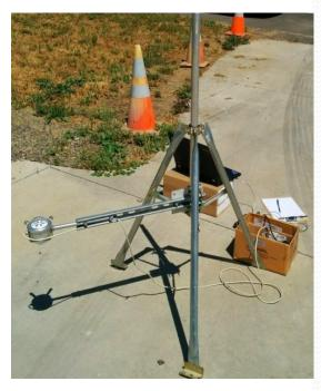
Albedometer with dual-pyranometer
